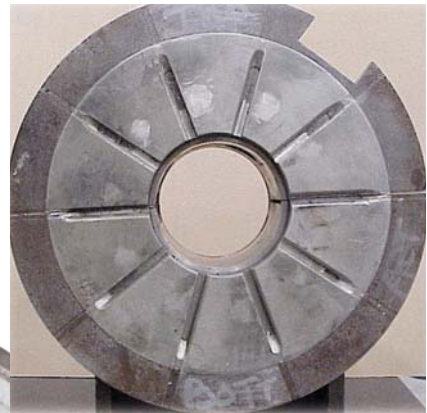
Figure 4 a (top): Active side bearing. Wear from misalignment of the thrust bearings. Source: TurboCare.
