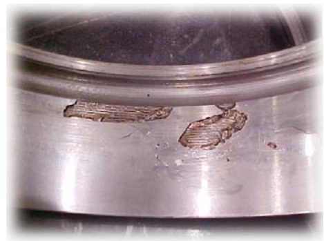
Figure 1: Babbitt failure due to poor bonding of the babbitt and the steel backing and fatigue. Source: TurboCare
