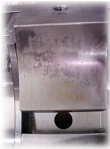
Figure 3: Triangular wear pattern from misalignment. Source: TurboCare
