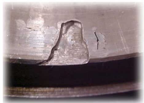
Figure 2: Fatigue from misalignment and high vibrations. Source: TurboCare
